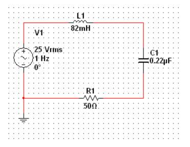
B. Energize the model and use the Multisim oscilloscope to measure the pharos currents and voltages across each element.
