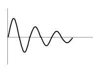
response concept in Chapter 1. When a sudden change is applied as the input, the sensor will produce decaying oscillations in the output. The response is characterized by a natural frequency of oscillation,  $f_N$ , and a decay constant,  $\alpha$
